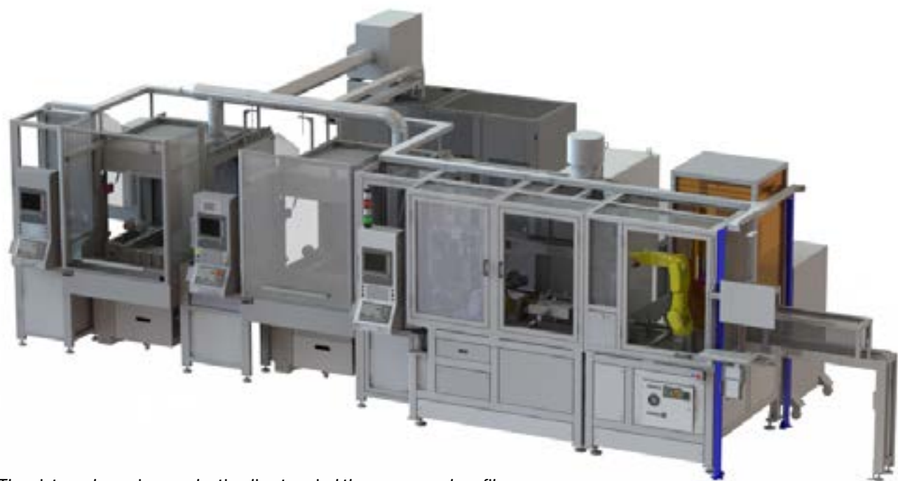
The picture shown is a production line to grind the groove and profile from turbo charger shafts
