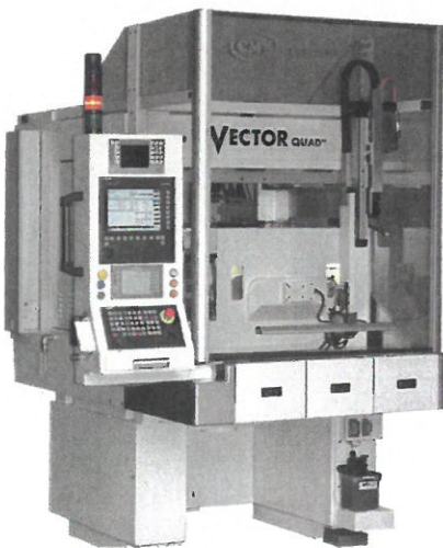
Double the output with the same footprint: a world first Vector Quad by CMT. Two workpieces ground simultaneously with automation in parallel giving a spark to spark time approaching zero
