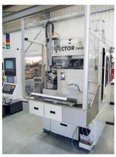
Grinding and loading therefore take place at the same time. The index time for the workhead drum is 1.2 seconds, giving a spark to spark time of less than two seconds.
