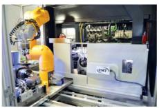
contained. The coolant is piped through the bottom of the guard and mist is removed either by an integrated extractor for conventional grinding. For high-speed grinding a separate unit having a higher capacity is used.
