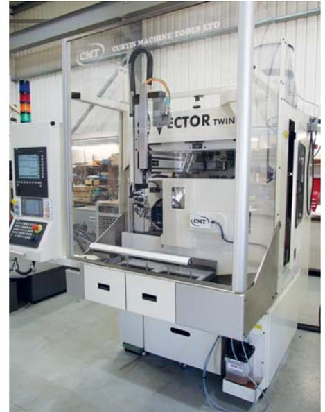
Grinding and loading therefore take place at the same time. The index time for the workhead drum is 1.2 seconds, giving a spark to spark time of less than two seconds.
